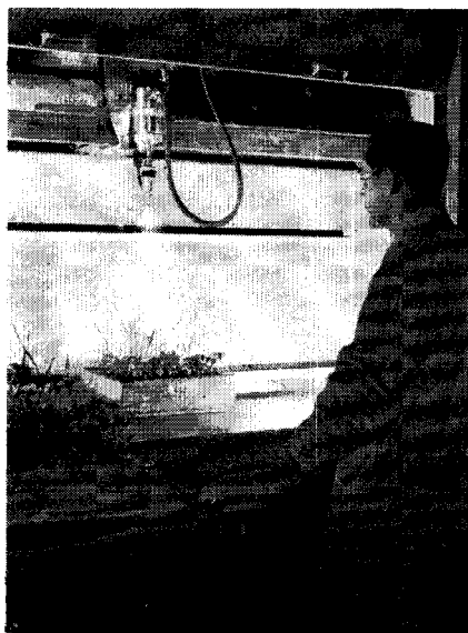
This moving sprayer can be adjusted to duplicate field spraying conditions
